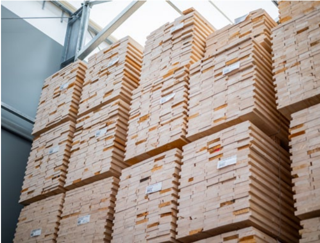
PEFC/06-34 -110-certified lumber stock is graded and sorted according to grade and surface quality.
