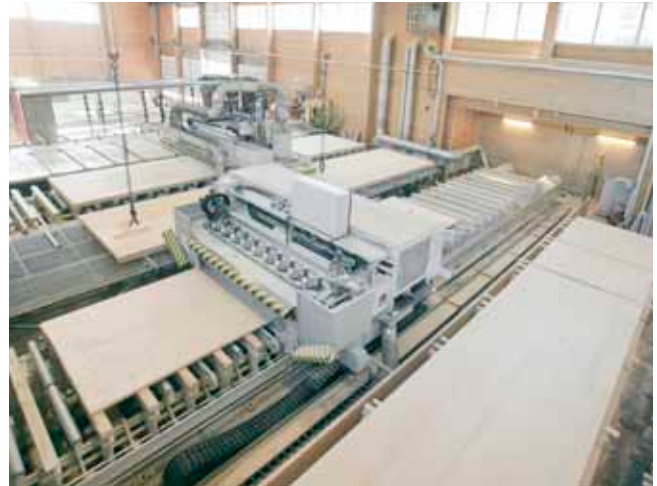
State-of-the-art CNC cutting machines facilitate both simple and highly complex patterns according to project requirements.
