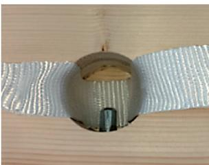
1. Insert the loop and dowel into the hole
