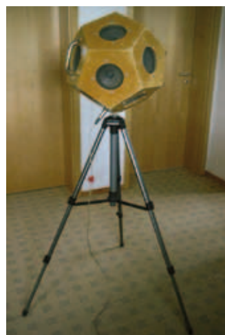
Fig. 19 – Dome loudspeaker as it is used in determining airborne sound insulation [7.14]
