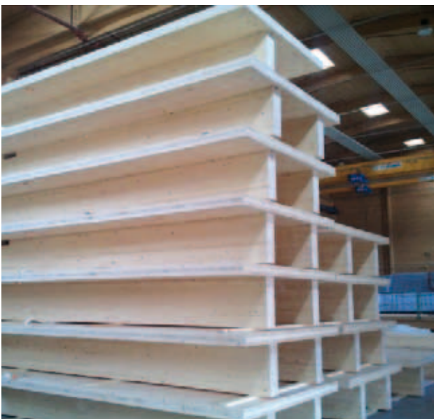
Finished rib elements, ready for transport
