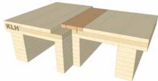
Fig. 7: Element connection with screw-connected top board
