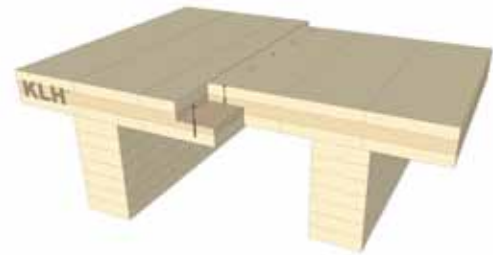
Fig. 6: Element connection with screw-connected stepped joint
