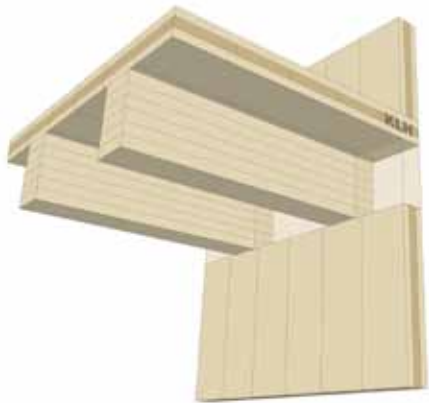
Fig. 9: Support of ribs at the wall element with suitable filling of the space in between
