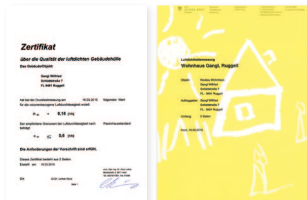
Fig. 6: A Blower Door Test in a passive house built with KLH® solid wood panels. Through the support of an excellent air tightness concept, an n_{50} -value of 0,15 h -1 could be realised [with the kind support of Eberle • d e n k f a b r i k • Dornbirn, Austria].
